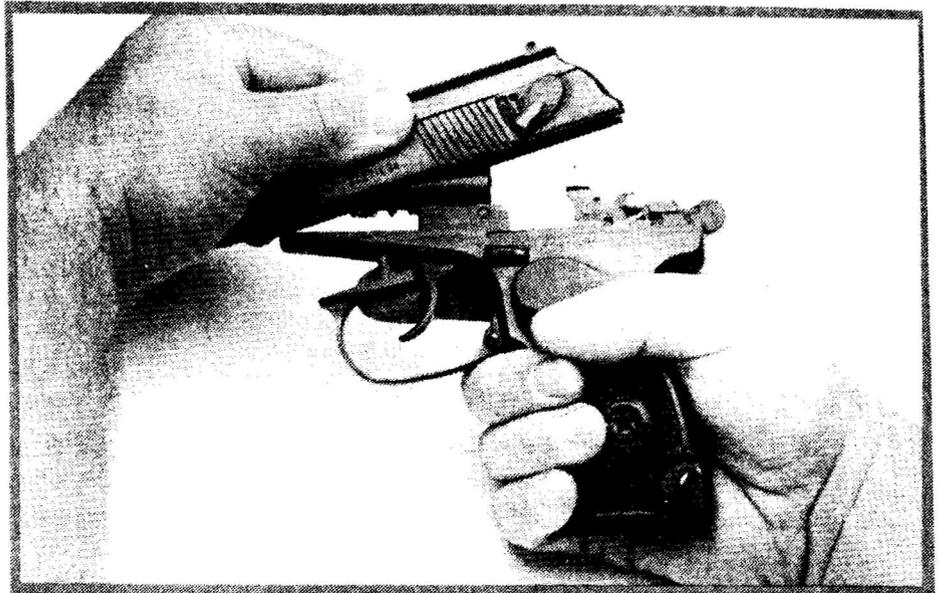
Holding the trigger guard in place with your trigger finger, draw the slide to the rear and lift upward until it comes off the frame.
