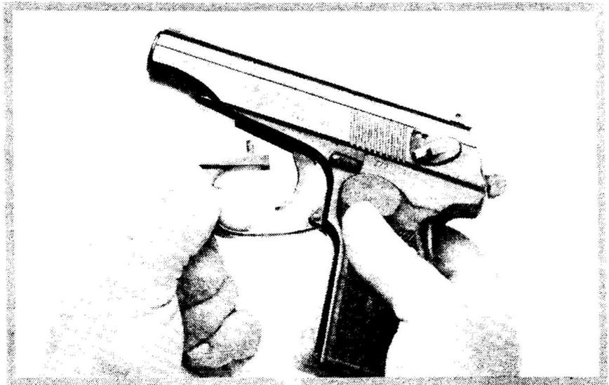
After ensuring that the pistol is unloaded, let the slide go forward. Leaving the hammer cocked, pull down on the front of the trigger guard and push it to the right or left.
