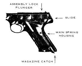
MAGAZINE. The magazine has an easily operable thumb-piece which facilitates loading. The magazine is held in the receiver by a magazine catch located at base of main spring housing. Thumb pressure on this catch releases the magazine.
